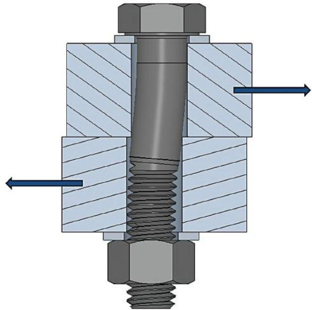
**Fig. 4 — Bolt bending when joint plates slip (image courtesy of Matrix Engineering Consultants).**
