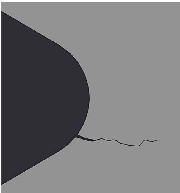
**Fig. 5 — Fatigue crack initiated near the thread root in a bolt (image courtesy of Matrix Engineering Consultants).**
