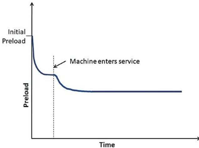
**Fig. 3 — Preload relaxation due to embedment vs. time (image courtesy of Matrix Engineering Consultants).**
