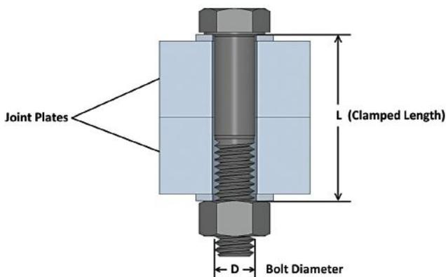
Fig. 1 — A bolted joint (image courtesy of Matrix Engineering Consultants).
