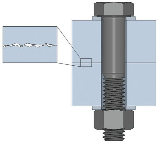
Fig. 2 — A bolted joint showing asperities on the surfaces of the joint plates (image courtesy of Matrix Engineering Consultants).
