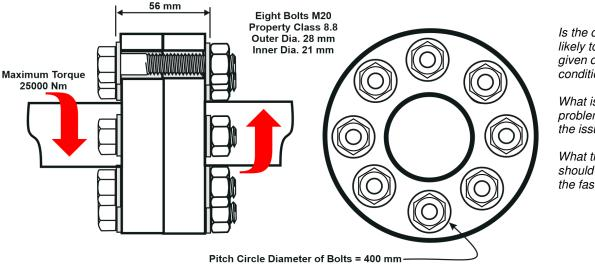
Is the drive joint shown likely to fail under the given dynamic loading condition?
