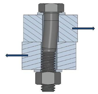
Fig. 4 — Bolt bending when joint plates slip (image courtesy of Matrix Engineering Consultants).
