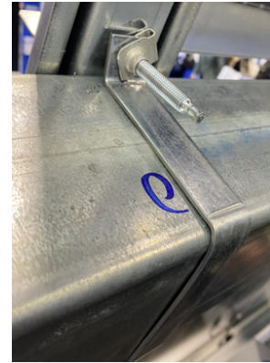
Figure 15. Clip-on nut used to mount torque
