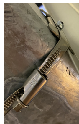
Figure 14. Hose clamp used on torque tube
