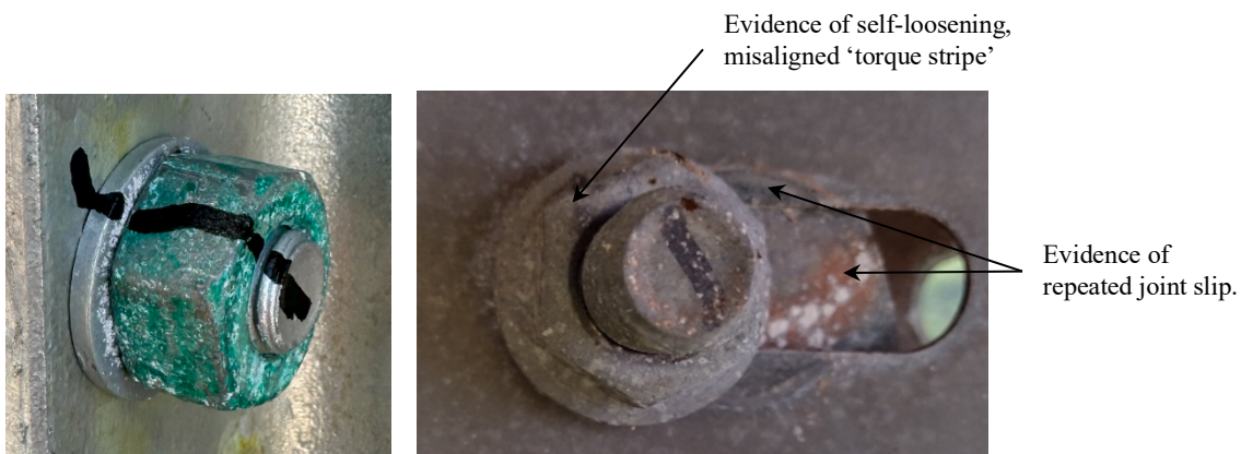
Image 24: Solar PV bolted joint with evidence of repeated joint slip and self-loosening.
