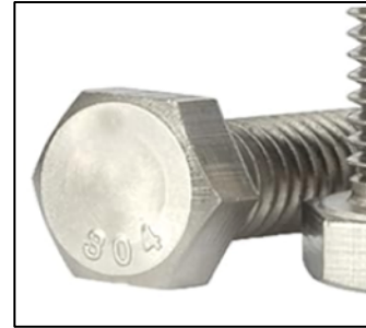
Figure 6: Fastener marked 304 only identifies the metallic composition, not the mechanical properties
