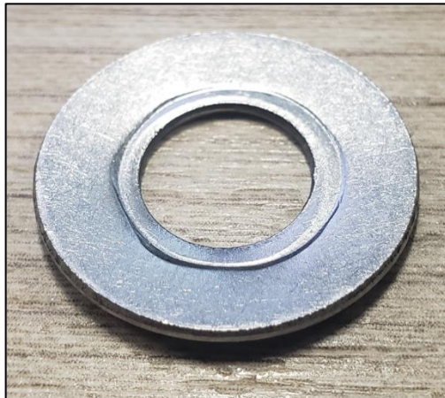
Figure 2: Evidence of compressive yield of a ‘soft’ washer tightened on a standard, round clearance hole.
